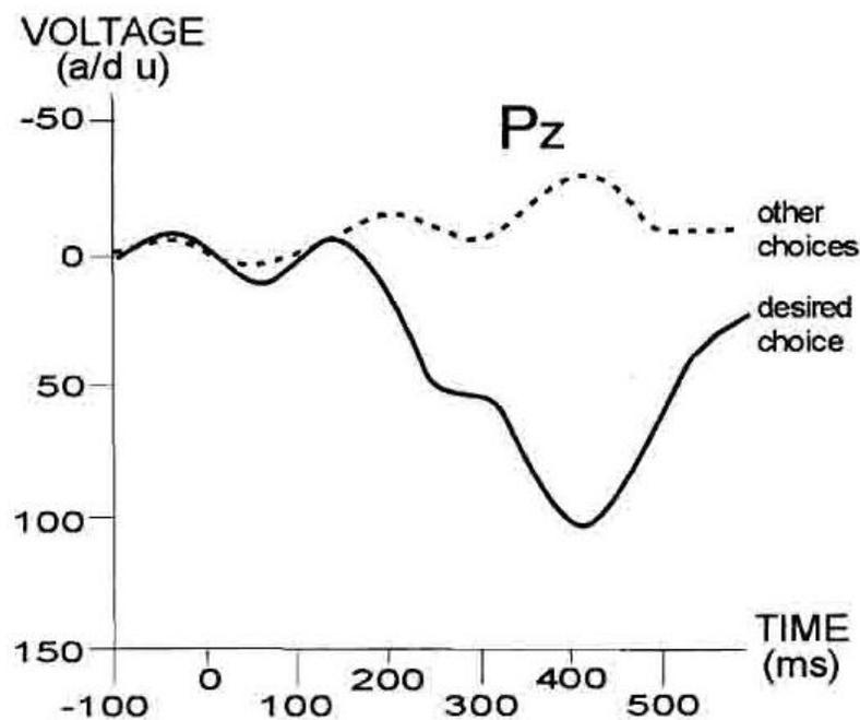
**Figure 2.** P300 BCI (modified from [23]). A matrix of possible choices is presented on a screen, and EEG is recorded from centro-parietal scalp while these choices flash in succession. Only the choice desired by the user evokes a large P300 [8, 10].
