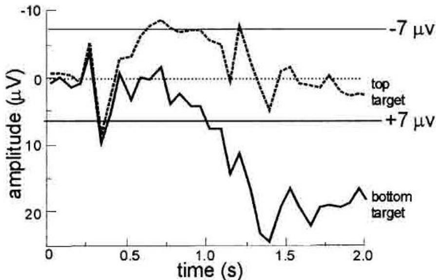
**Figure 1.** Slow Cortical Potential (SCP) BCI (modified from [23]). Scalp EEG is recorded from the vertex. Users learn to control SCPs to move a cursor towards a target at the bottom (more positive SCP) or top (more negative SCP) of a computer screen [4, 5, 23].
